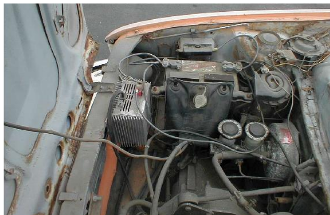
The right side has the car battery and the 120v-12V converter to keep the car battery charged. I put in a power brake master cylinder.
