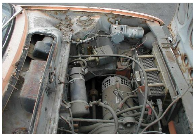
The left side has the vacuum pump so the brake booster works. There is a PVC reservoir for the vacuum on the firewall. The big box below to the left of the pump is the vacuum switch.
