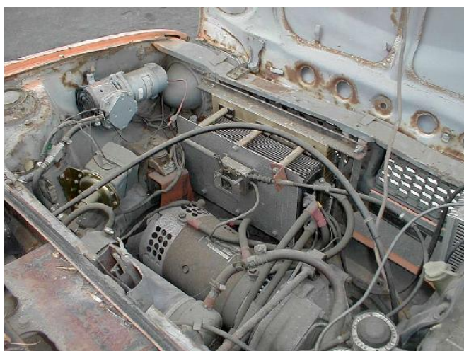
The controller heat sink behind the grill.
