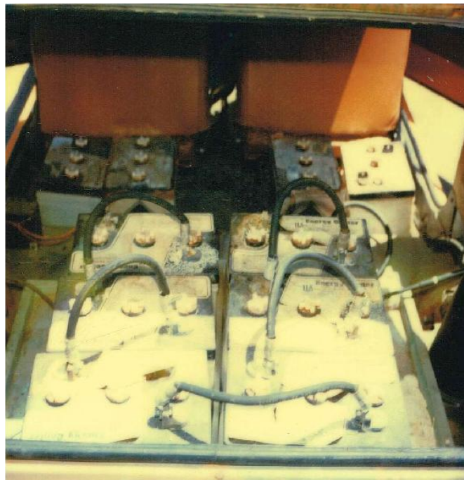
Original 6-V batteries weighing down the back.
