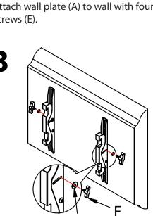
Turn two handles (F) into the mounts through washers (G) but do tighten. After wall mounting your TV, adjust TV to the desired viewing angle and turn to tighten both handles.
