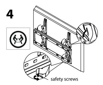
We strongly recommend two people, one on each side, hold the TV. Tilt the top of the TV toward the wall. Carefully position TV mounts (B and C) over the wall plate until both lock in place. Tighten safety screws.
