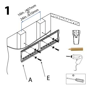
This mount is designed to be attached into wood studs. DO NOT use wall anchors. Using a stud finder, find the center of two adjacent studs. With a pencil mark the hole locations at the desired height, making sure you are level. Use the wall plate (A) as a template to mark the two remaining hole locations. Drill pilot holes at four pencil marks 2.5 in. (64 mm) deep, using a 7/32 in. or 5.5 mm diameter drill bit.
