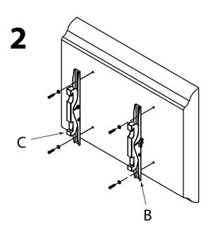
Attach TV mounts (B and C) to the TV back panel. Make sure to select the same height screw holes, so the mounts are centered and level.
