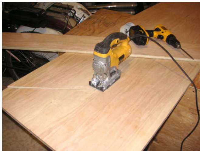
A jig saw worked much better where the circular saw cuts met..
