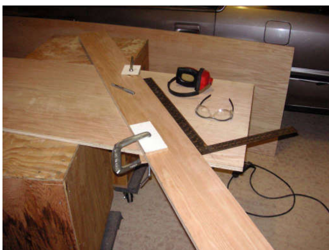
I used factory edges as a straightedge that I clamped to work piece. I just adjusted the line for the offset of the saw base.
