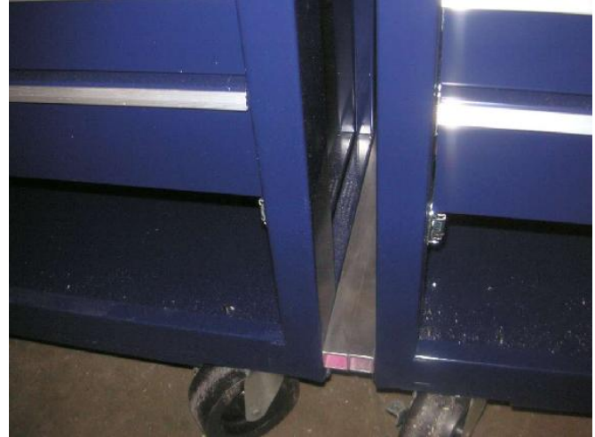
The tubes space the casters apart so the don't clang into one another as you roll it around.
