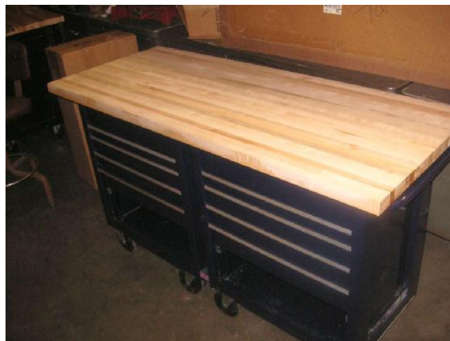
Here is the whole top. Note bottom drawers still out where I bolted the two boxes together.
