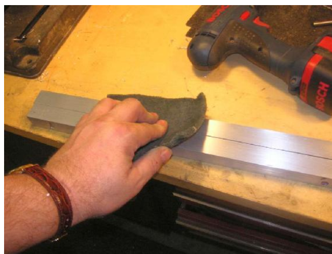
A Scotchbrite pad put a nice satin finish on the aluminum tubes. The Bosch drill had its charger fail and it got tossed soon after this project.
