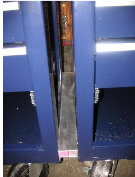
The tubes space the casters apart so the don't clang into one another as you roll it around.
