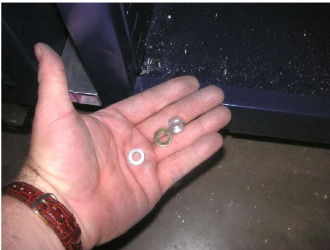
A flat-washer under the bolt and the nut spreads the load. Use a lock-washer to keep things tight.
