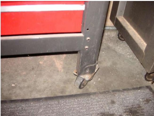
The casters on the old workbench reveal how lightweight and cheap it is.
