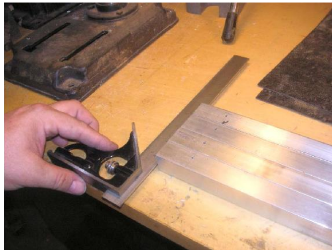
Make the ends and holes all line up. I am building two workbenches, so four tubes.
