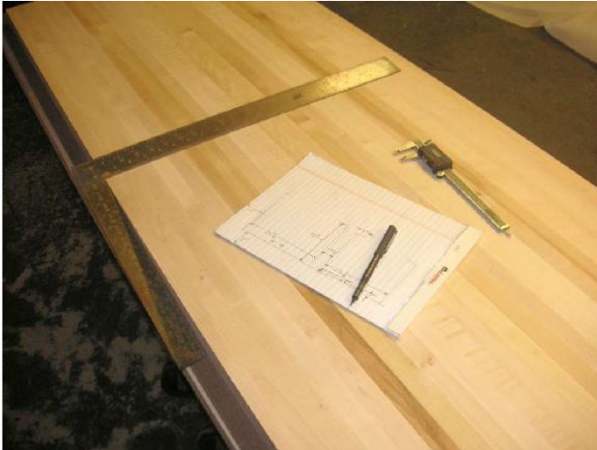
The square helped with the layout. The caliper set the depth of the router bit.
