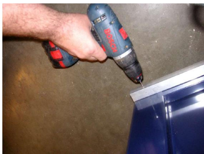
The holes are still smaller diameter pilot holes. Use them to drill pilot holes in the toolboxes. It would have been smarter to clamp the tube to the box, but I was in a hurry.
