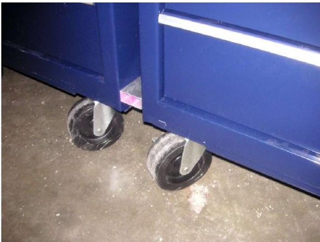
The new workbench has casters that can take a lot of weight. They roll much easier as well.
