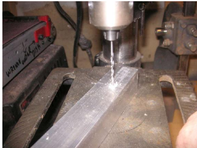
Drill the tubing in a press to keep the holes square. The bolts have to line up.
