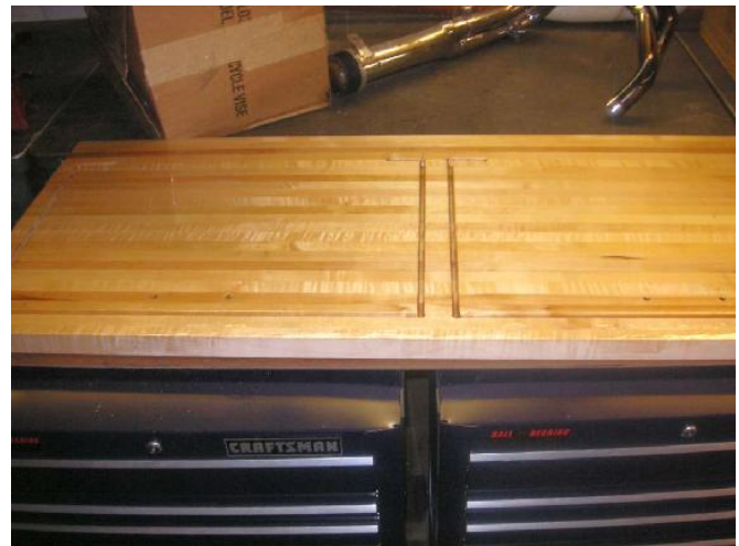
Now you can mill slots in the underside of the top to fit the toolboxes.
