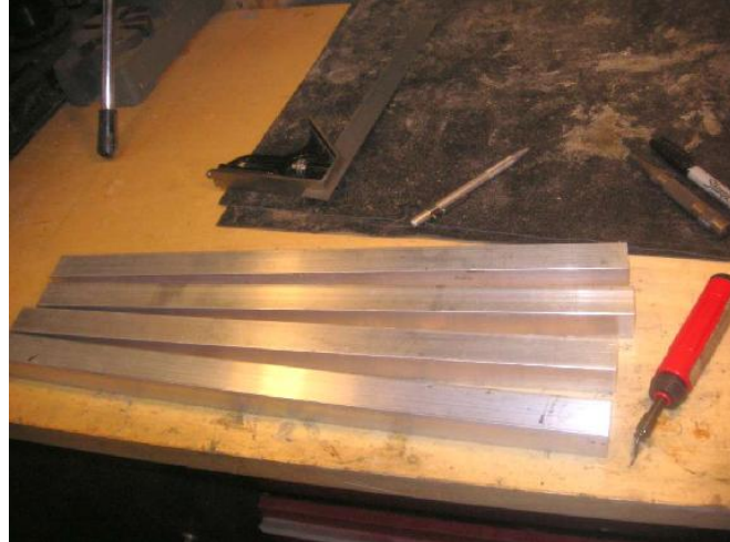
I used Home Depot aluminum tubing to connect the two toolboxes together at the base.
