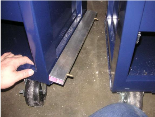
The tube slip on, especially if the holes are a bit oversize. I go 1/32nd over, or 11/32 drill.
