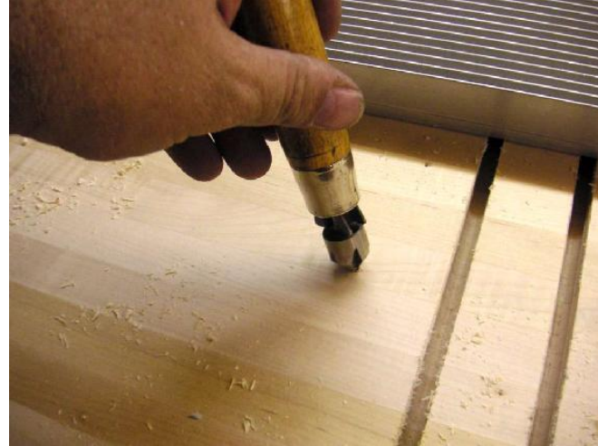
I deburred the holes despite deciding to not screw the top down. Its weight keeps it put.
