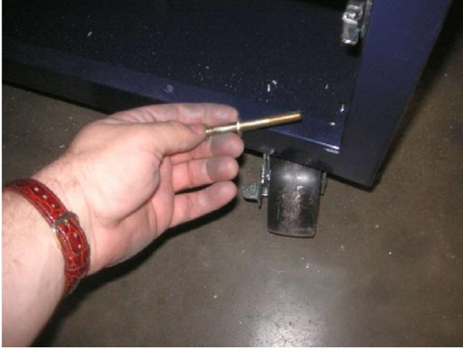
The 5/16th bolt slips in at a strong structural place in the toolbox frame.
